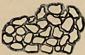
FIG. 12. Water Film surrounding Soil Particles.
